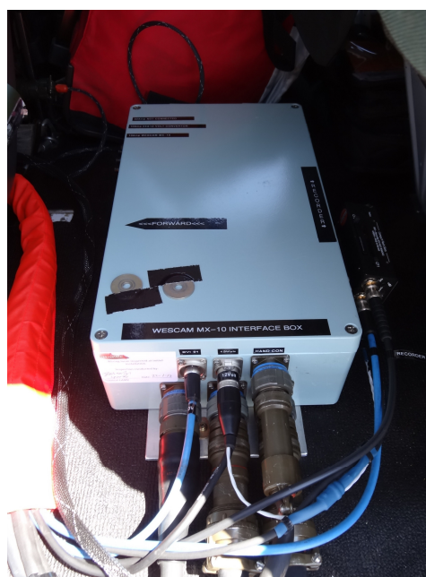
MX10 Interface Box Fitted to FB302
